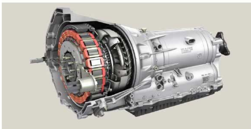
Figure 7: The 8P70H transmission with the Electric Motor.
